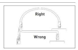
When routing hose line, provide a smooth bend radius. Avoid sharp bends which may cause hose to collapse and restrict flow.
