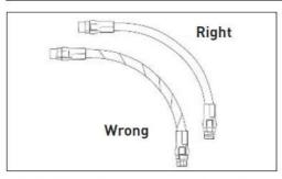
1. Avoid twisting hose when installing.
