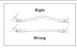
2. Allow some slack in assembly for changes in length that occur under pressure.
